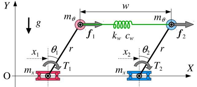
Fig. 1. Coupled inverted pendula (CIP) model with viscoelastic connection.
