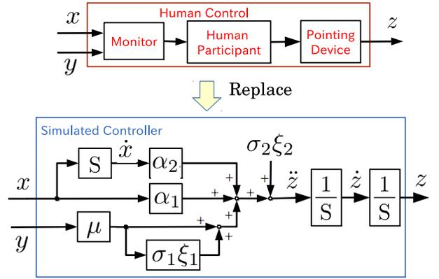
Fig. 3. Tracking control module.
