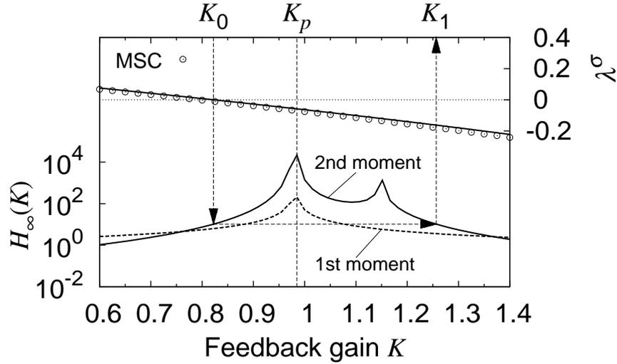
FIGURE 6. Lyapunov exponent  $\lambda^\sigma$  and  $H_\infty$  norms as functions of the mean feedback gain  $K$  for  $\sigma = 1$ .
