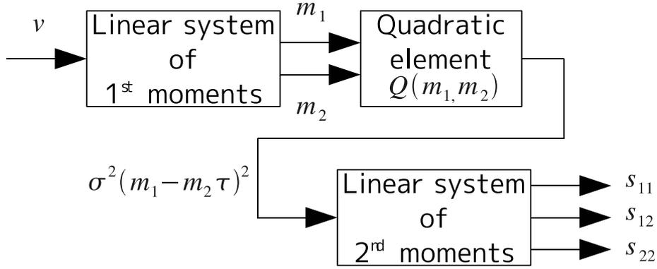
FIGURE 1. Block diagram of MDE
